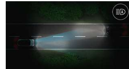
automatic main/dipped beam headlight activation. This system works using a camera that analyses light flows based on lighting and traffic conditions.
