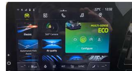
eco mode. This function makes the car as environmentally efficient as possible. It acts upon certain power consuming systems in the vehicle (heating, air conditioning, power-assisted steering etc.) and on certain driving actions (acceleration & gear changing).
